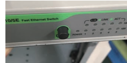
LED ON/OFF switch: popped out
