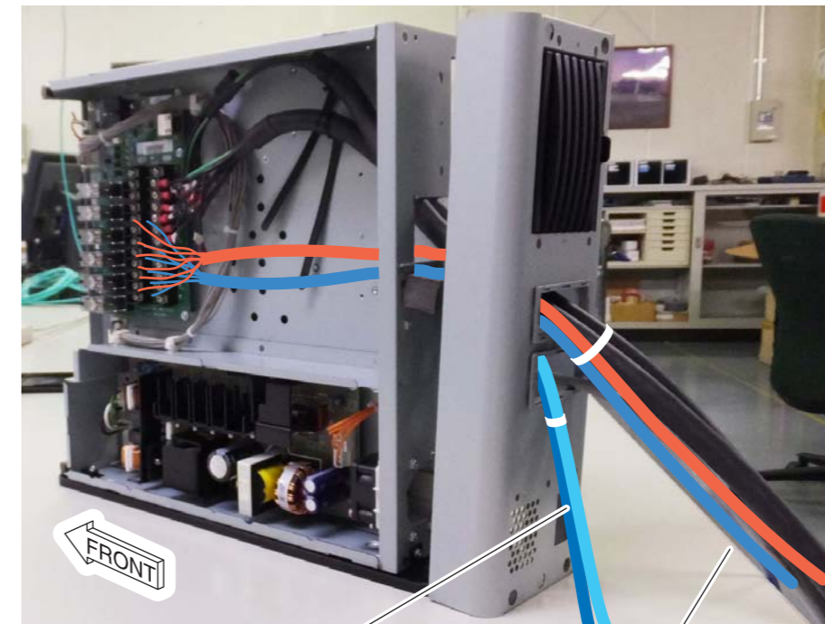
LAN cable (between MP and MC) LAN cable (between MP and AP) X-Ray shot cable(s) and the bucky cable(s)
